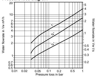
Pressure loss diagram with open valve at 20°C. The values indicated are applicable to spring loaded valves with horizontal flow. With vertical flow, insignificant deviations occur only within the range of
