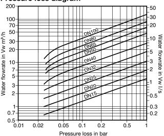
Pressure loss diagram with open valve at 20°C. The values indicated are applicable to spring loaded valves with horizontal flow. With vertical flow, insignificant deviations occur only within
