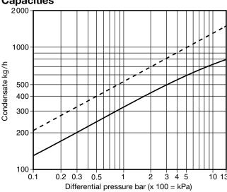
Hot water capacity —— Cold water capacity — –
